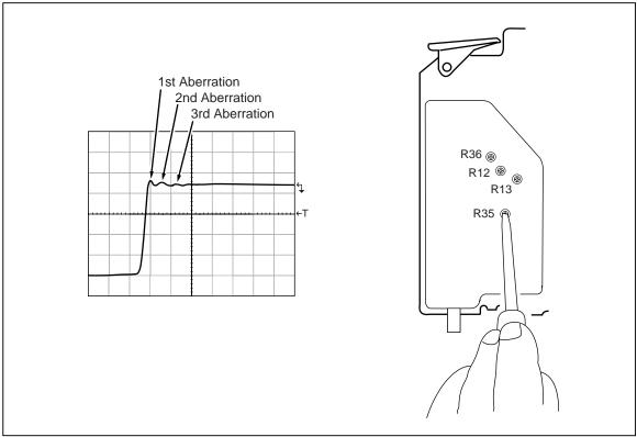
Figure 17. Adjusting Edge Aberrations
