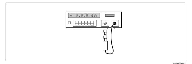
Figure 11. Connecting the HP 437B Power Meter to the HP 8482A or 8481D Power Sensor
