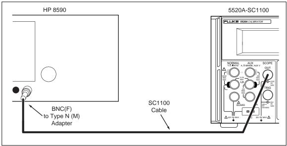
Figure 9. Leveled Sine Wave Harmonics Verification Setup
