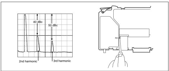
Figure 16. Adjusting the Leveled Sine Wave Harmonics
