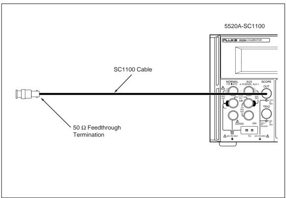
Figure 14. Overload Function Verification Setup
