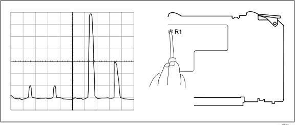
Figure 15. Adjusting the Leveled Sine Wave Balance
