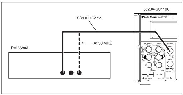
Figure 6. AC Voltage Frequency Verification Setup
