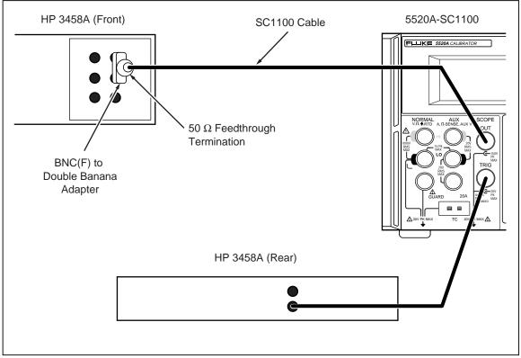
Figure 2. Equipment Setup for SC1100 Voltage Square Wave Measurements
