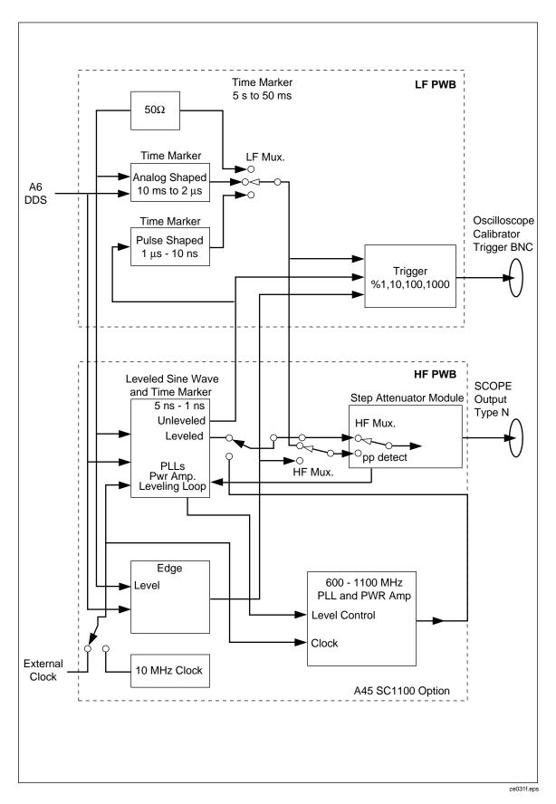
Figure 1. SC1100 Block Diagram
