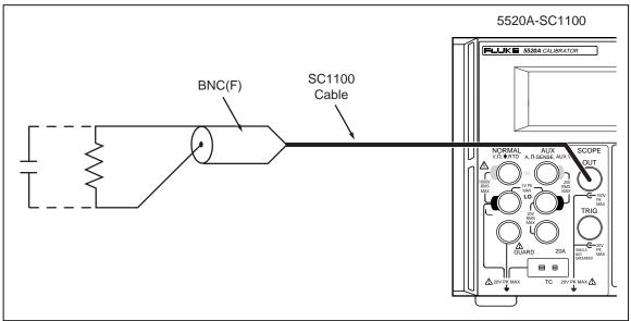
Figure 5. MeasZ Function Calibration Setup
