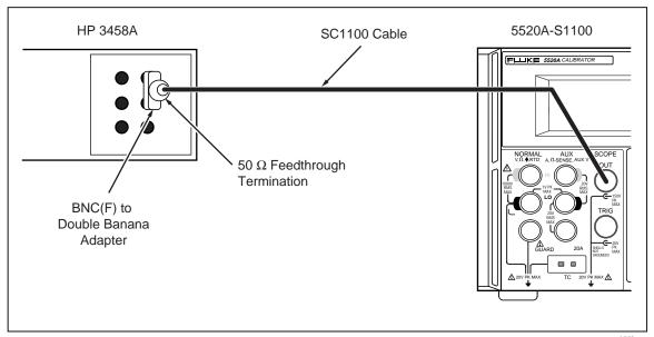
Figure 3. Equipment Setup for SC1100 Edge and Wave Gen Square Wave Measurements.
