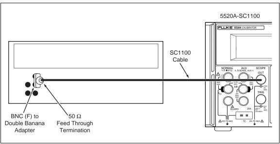
Figure 13. Wave Generator Verification Setup
