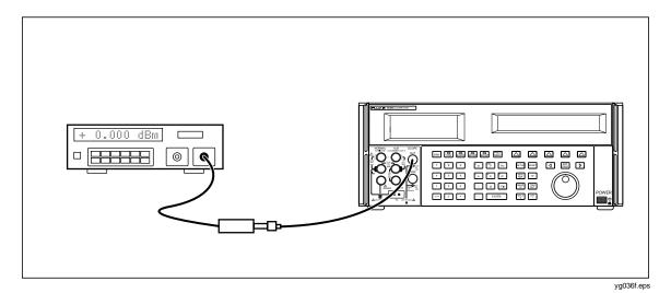
Figure 12. Connecting the Calibrator to the HP Power Meter and Power Sensor
